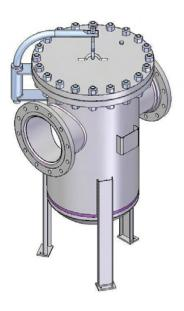
PAP Pot / Bucket / Basket strainers have been specifically designed to meet all customer requirements including high pressure applications. Designed and fabricated according to ASME VIII Div.1 as standard version, they can also be supplied according to other pressure vessel regulations. I.e. ASME B31.3 etc.
